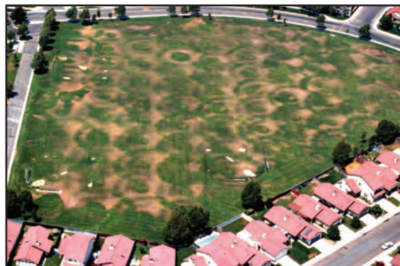
Figure 12 - Aerial view of sports field with severe 'donuts' caused by rotary sprinklers.
