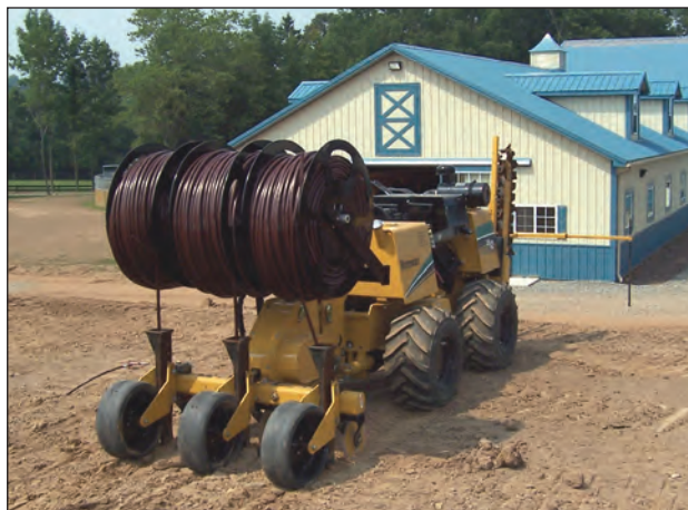
Figure 31 - A Vermeer® LM42 laying Netafim dripline three rows at a time.
