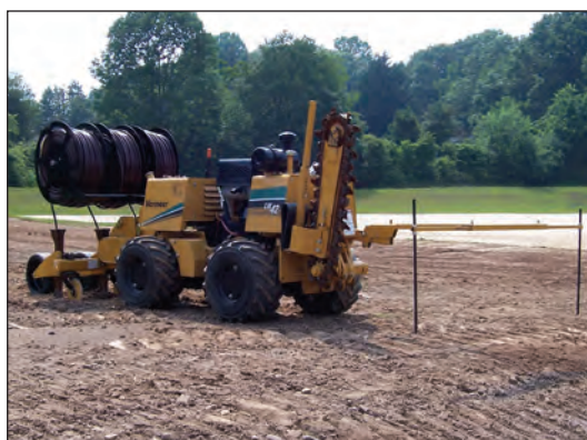
Figure 35 - Vermeer® LM42 shown with 3-blade vibratory plow. Standard tubing rack not shown on picture at right.
