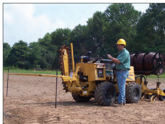
Figure 35 - Vermeer® LM42 shown with 3-blade vibratory plow. Standard tubing rack not shown on picture at right.
