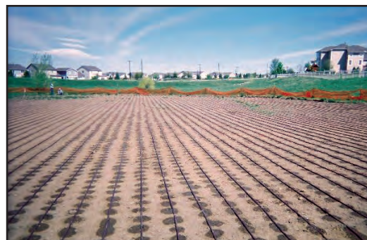
Figure 30 - Examples of wetted pattern of Techline CV after running for four minutes and prior to being covered with topsoil.
