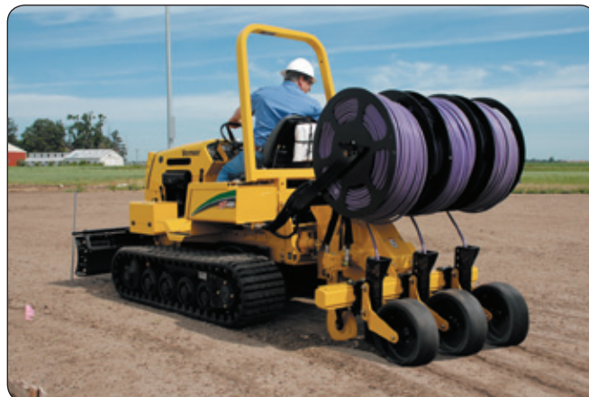
Figure 18 - MB-40 Can Be Mounted on the Vermeer® RTX-450. This ride-on unit is excellent for large installations.
