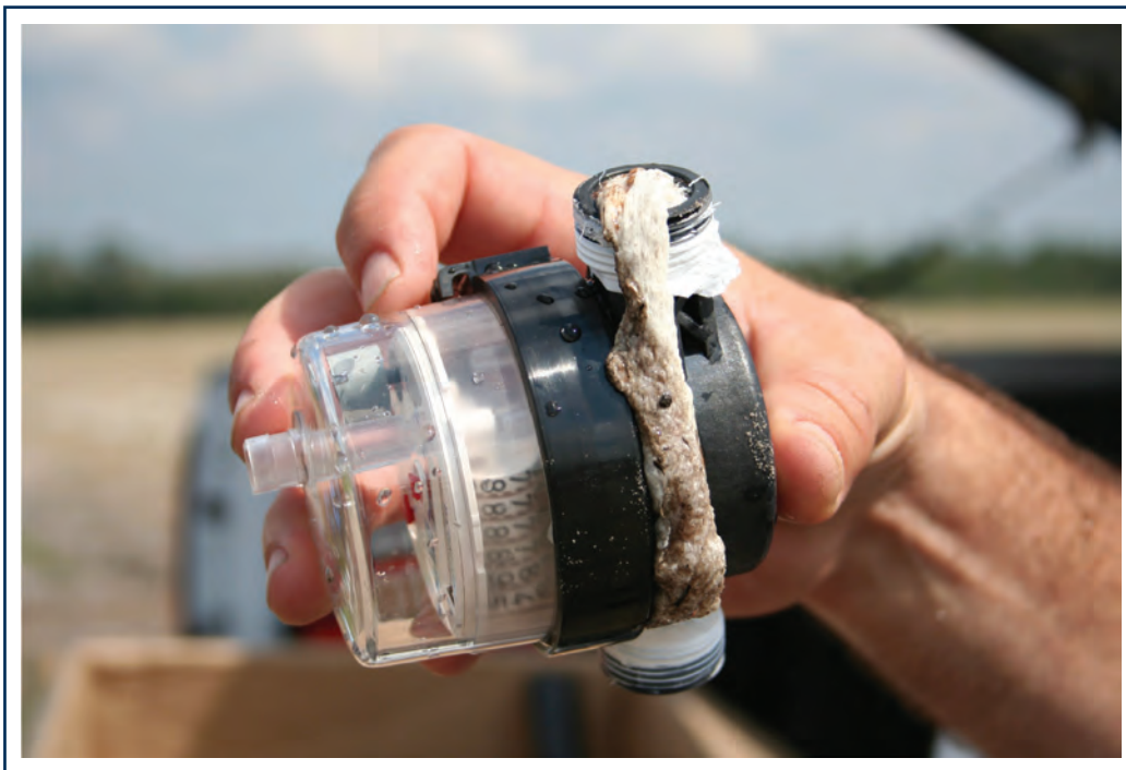
FIGURE 16. Filamentous sulfur slime completely clogging a small water meter
