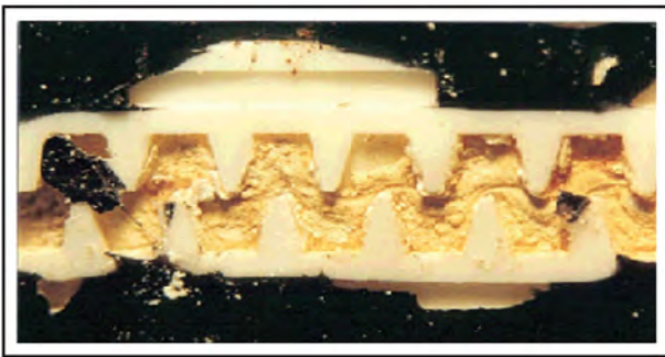
Figure 7.1. Dripper with calcium precipitate. The black pieces in the picture are pieces of the cut-away plastic dripperline and not contaminants.
