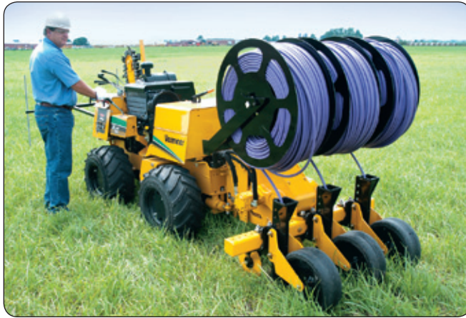
Figure 15 - The MB-40 Multi-Blade Vibratory Plow. Shown here with three 1,000' rolls of Netafim Bioline® attached to the versatile Vermeer® LM-42 power unit. This unit has a variety of attachments and fits into narrow areas.
