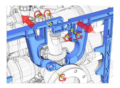
4. Disconnect the vertical beams by releasing the bottom screws on each corner.
