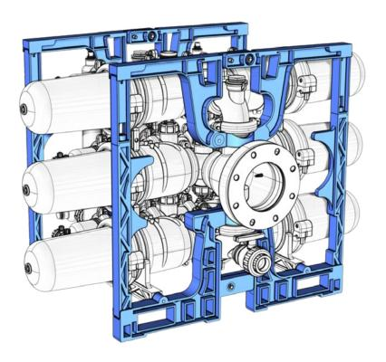
3. Disconnect the three screws and separate the horizontal beams.
