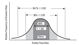
Both the 'X' and 'Cv' are integral parts of the Emission Uniformity equation which describes uniformity due to manufacturing design and variation. This equation does not consider the possible disuniformity that may occur from emitter plugging:
