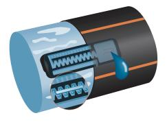
require over 200 mesh. In addition, the raised inlet to Netafim's drippers prevents plugging from settled debris in dripline products.
