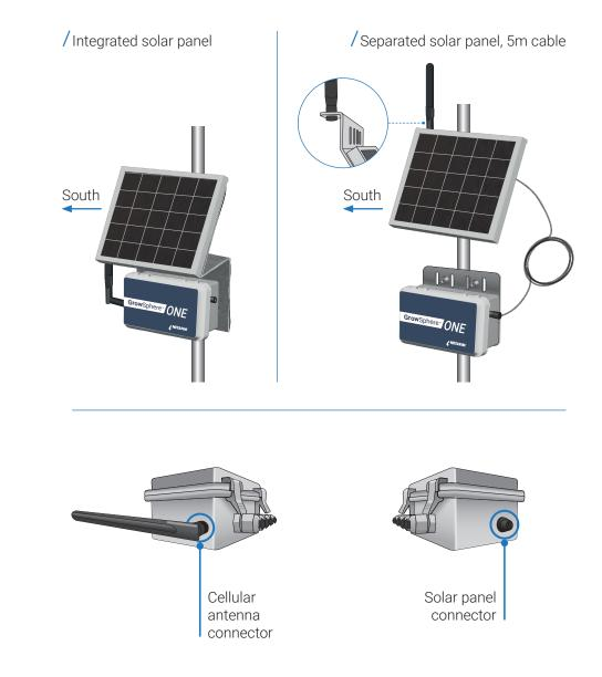
\* Stay updated with your Netafim representative for sensor compatibly. \*\* The unit is provided with a SIM card /Prior to configuration, ensure the unit is charged for a minimum of 5 hours, by using the provided charging cable (as demonstrated in the diagram below). After charging, disconnect the cable and connect the solar-panel cable instead
