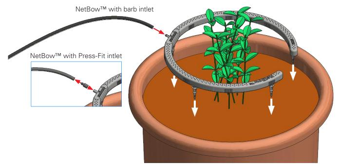
• Adjust the NetBow<sup>™</sup> inlet T orientation (up/down) as to allow the optimal micro-tube position.
