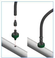
• PCJ with Press-Fit outlet and elbow Press-Fit to barb adaptor
