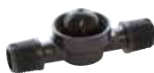
TLCV Inline Check Valve • Flow Range: 0.9 to 4.4 GPM • Opening Pressure: 10.2 psi • Closing Pressure: 5.8 psi (13.4 Feet Column of Water)
