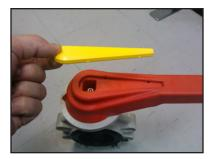
**STEP 2:** Remove the bolt under the yellow insert with a 5mm Allen key. Once the bolt is removed, the handle can be separated from the valve.
