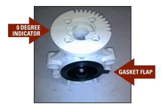
**TIP 4:** When installing the shaft, the square end of the shaft must be oriented at the top of the valve body. Notice the groove at the top of the shaft (square end). This groove needs to be on the opposite end from the gasket flap. See pictures below.
