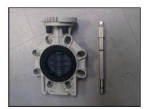
**STEP 5:** Remove the disc. The disc can usually be pressed out by hand. If it does not release easily, carefully tap it free with a rubber mallet.
