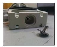
**STEP 4:** Remove the shaft. The shaft exits from the top of the valve body. Push on the bottom of the shaft using a screwdriver to free it up.
