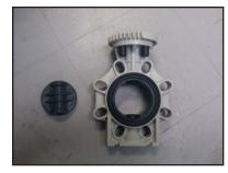
**STEP 6:** Remove the top plate. After removing the protective caps, use a 13mm wrench to remove the nuts. Once the bolts are free, the top plate can be separated from the body.
