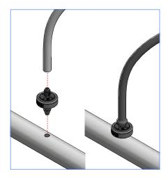
PCJ with Press-Fit outlet and straight Press-Fit to barb adaptor
