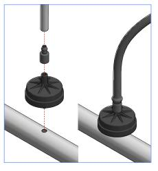
• PC with Press-Fit outlet and elbow Press-Fit to barb adaptor
