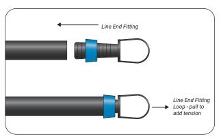
Figure 4: Space-It Dripline with line end fitting.
