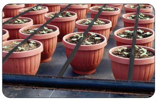
**Figure 1:** Polyethylene pipe supply header with Space-It Dripline.
