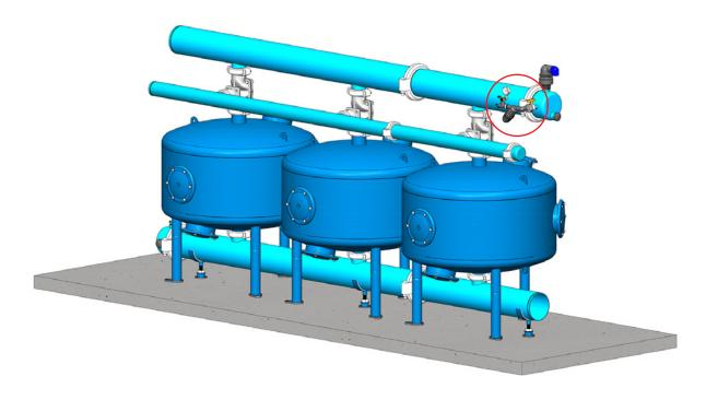
14. Place the stand of the backwash controller so that it is close to the control assembly (make sure it meets your needs for both operation and maintenance). Secure it to the concrete slab with 10 mm spreading anchor bolts.
