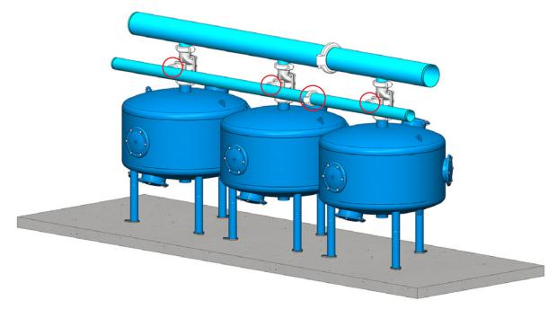
5. Connect the outlet manifold to the outlets of the tanks and the outlet manifold sections to each other with grooved couplings.
