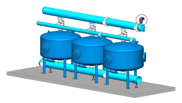
**12.** Connect the air valve to the socket on the top of the inlet manifold end-cap.
