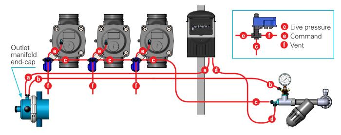
17. Connect the solenoids to the BackFlush controller expansion cards ordered in sequence, from left to right. Red wire = + / black wire = common (inversing wire polarity will change NC to NO).
