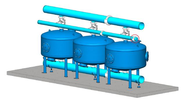
**8.** Connect the end-cap to the inlet manifold with a grooved coupling. Make sure that the end-cap is placed with the socket for the air valve pointing upwards and the socket for the control assembly pointing sideways.
