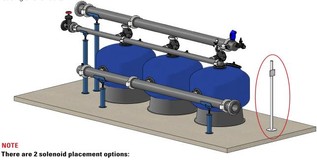
A. All the solenoids are placed on the solenoid bracket on the controller stand.B. Each solenoid is placed on its respective backwash valve.
