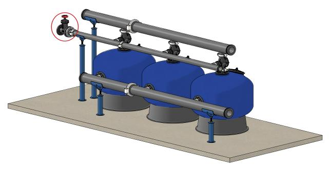
8. Connect the end-cap to the backwash manifold with a grooved coupling.
