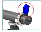
c. Connect the control assembly to the socket on the side of the inlet manifold end-cap.
