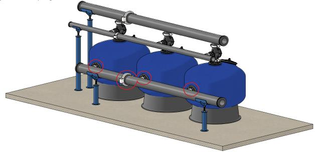
**6.** Check and confirm that the position of the system is where it should be relative to the inlet and outlet main pipelines.
