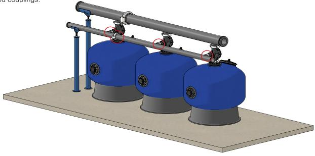
**5.** Connect the outlet manifold to the outlets of the tanks and the outlet manifold sections to each other with grooved couplings.
