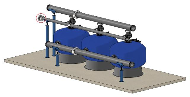
**b.** Connect the backwash flow-control valve to the flange adaptor.
