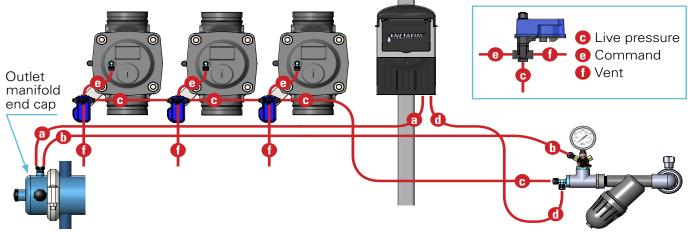
**20.** Connect the solenoids to the BackFlush controller expansion cards ordered in sequence, from left to right. Red wire = + / black wire = common (inversing wire polarity will change NC to NO).
