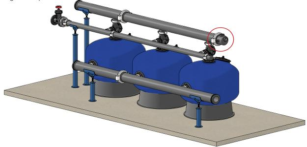
**b.** Connect the air value to the socket on the top of the inlet manifold end-cap.
