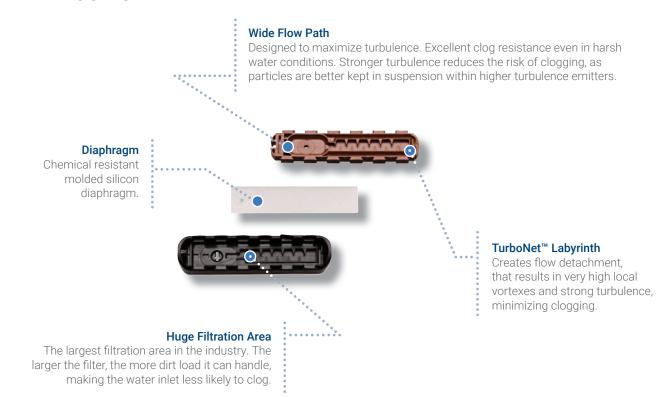
**Designed Specially for Subsurface Drip Irrigation Application** with mulitple levels of built in protection against clogging.
