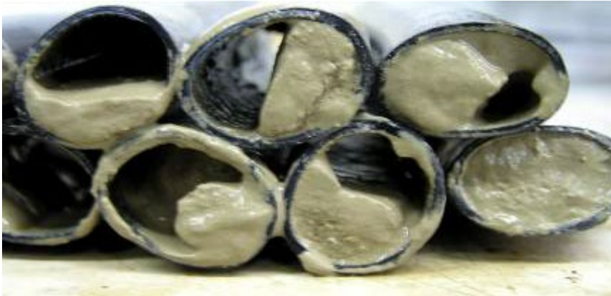
Clogging of driplines from physical factors
