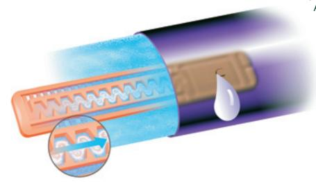
Netafim USA's thinwall dripperlines. A flap over each dripper outlet systematically opens and closes during start-up and shut-down, providing uninterrupted flow while open and protection against soil ingestion and root intrusion when closed.
