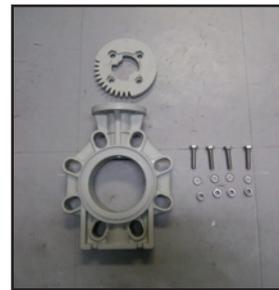
**STEP 7:** Remove the bushing. The bushing exits through the top of the valve body. Use your thumb to push the bushing upward so it can be removed from the valve body as pictured below.
