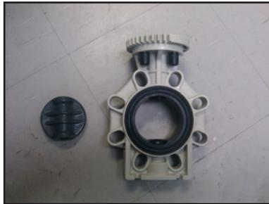
**STEP 6:** Remove the top plate. After removing the protective caps, use a 13mm wrench to remove the nuts. Once the bolts are free, the top plate can be separated from the body.
