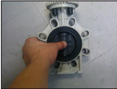
(Use caution to not damage the threads on the shaft when removing)
