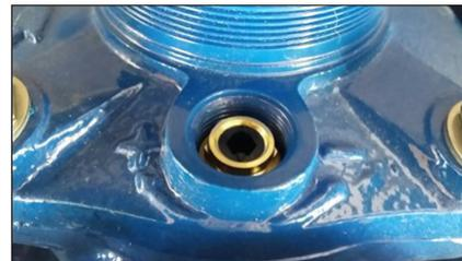
FIGURE 2 - The seal and calibration bolt have been removed revealing the calibration set screw.
