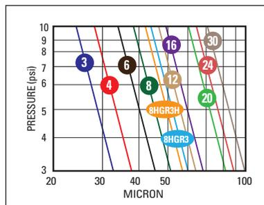
FIGURE 3 - Particle size separation
