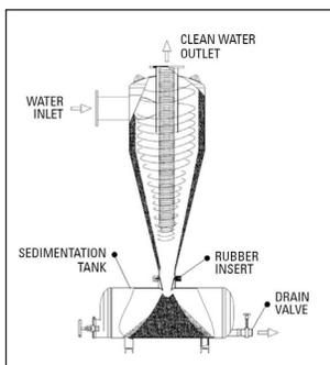
FIGURE 2 - Function and components of a Hydrocyclone
