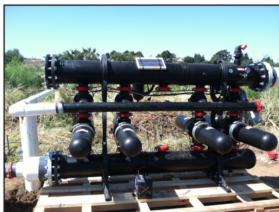
Figure 2. Example of a Netafim Apollo Disc-Kleen Filter
